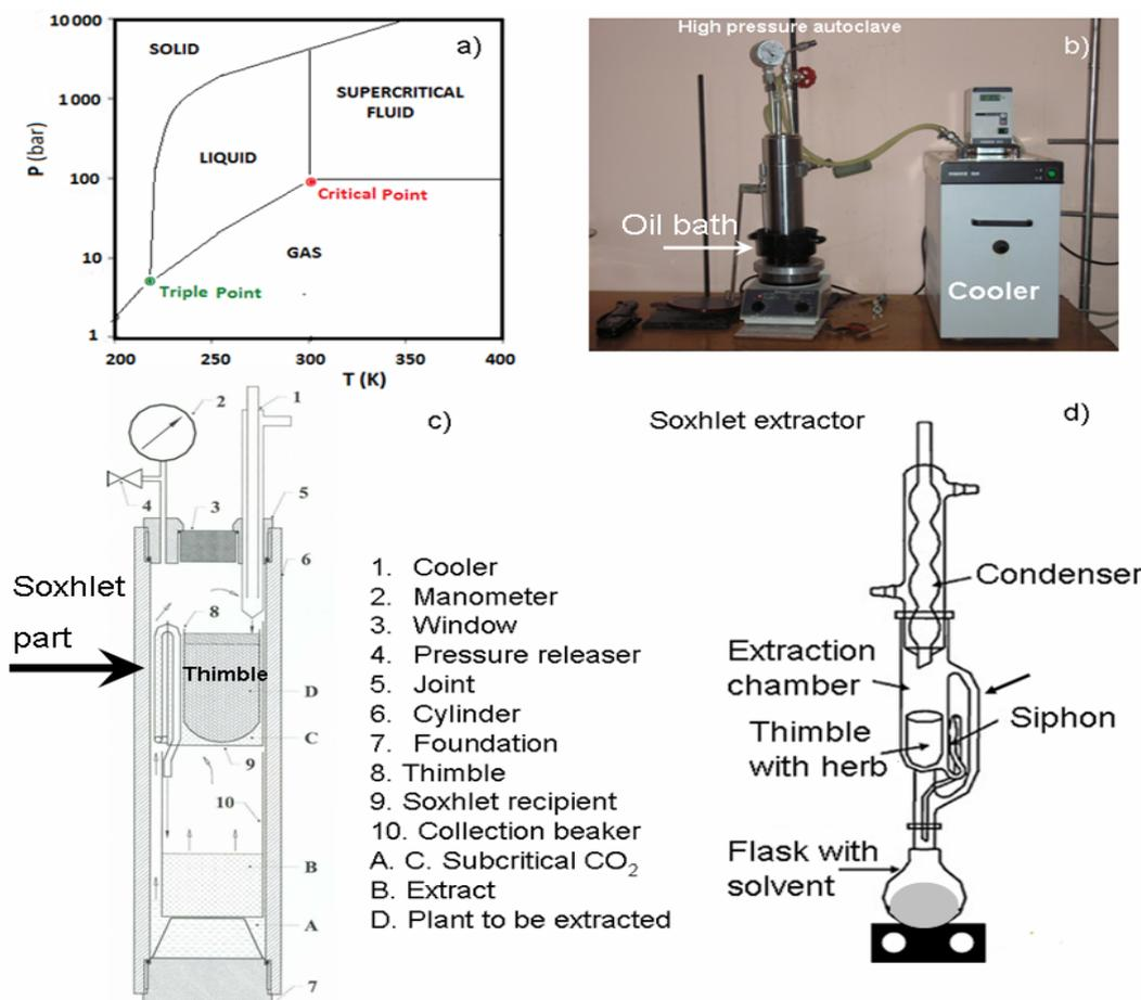
**Figure 1.** a) Phase diagram of carbon dioxide. b) Photo of autoclave for CO<sub>2</sub> extraction. c) Scheme of the internal part of the autoclave including the Soxhlet extractor d) Scheme of the Soxhlet extractor.
