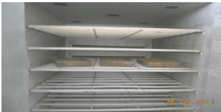
Figure 1. Laboratory kiln for the removal of mechanical humidity with the temperature 105-110C
