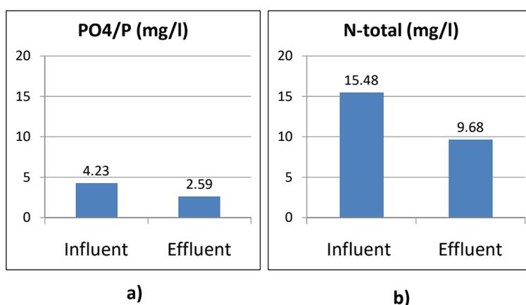
**Figure 4.** The mean values of influent and effluent wastewater  $\text{PO}_4\text{-P}$  (a) and N-total (b) concentrations
