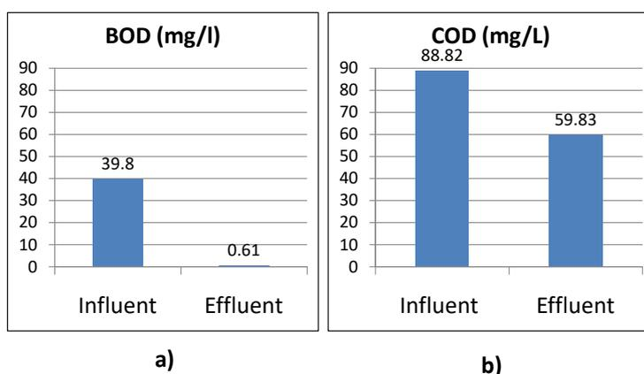
**Figure 3.** The mean values of influent and effluent wastewater BOD5 (a) and COD (b) concentrations
