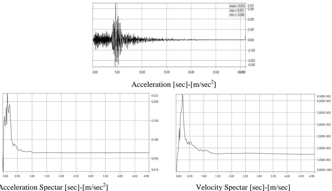
**Figure 3.** Time history obtained from Istog Earthquake recorded at location station PEJA, component N
