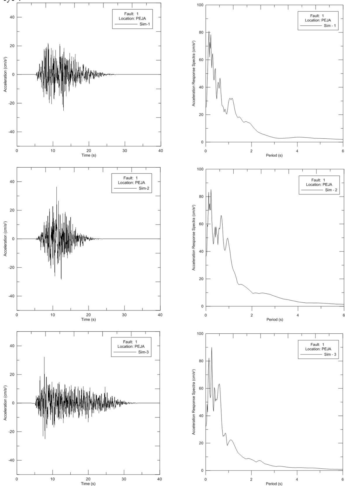
**Figure 2.** Simulated accelerations from Fault -1 to location PEJA, distance 30 km Max Magnitude 6.1
