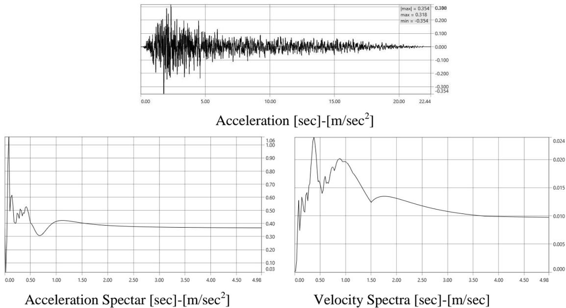
**Figure 4.** Synthetic Time History, acceleration and velocity spectra for location Peja, componente N
