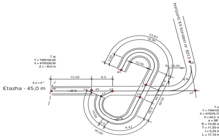
**Figure 3.** Schematic view of spiral ramp in one level (-45,0m)
