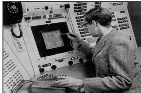
**Figure 4.** In the first half of the 1950s a drawing with a light pen on the screen (TURKCADCAM, 2011)
