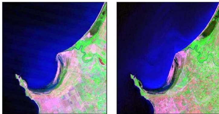
Figure 7. June 1992 July 2002 .Colour composition (bands 742=RGB) from Landsat images of 1992 and 2002 in the coastal sector between Pali Cape–Erzeni River embouchure. The image covers a 12x12 km
