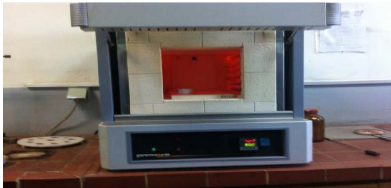
Figure 1. Laboratory furnace at a temperature of 800-1000°C
