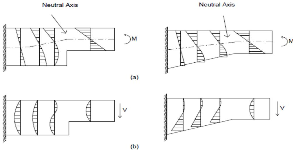
**Figure 3.** Stress distribution on non-prismatic elements a) Normal stress due to only bending moment
