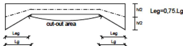
**Figure 5.** Linearly haunched elements modelling
