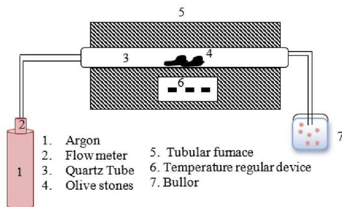
**Figure 3.** Schematic diagram of the apparatus (Spahis et al., 2008)
