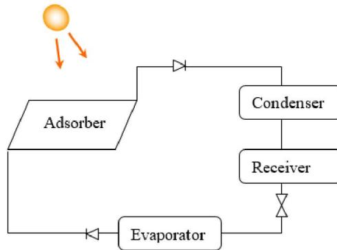
**Figure 1.** Schematic diagram of simple solar adsorption refrigerator
