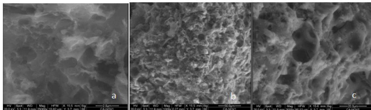
**Figure 4.** SEMs of (a) no impregnated olive stones, (b)olive stones impregnated by  $ZnCl_2$  (7.35 mmol/g), (c) olivestones impregnated by KOH
