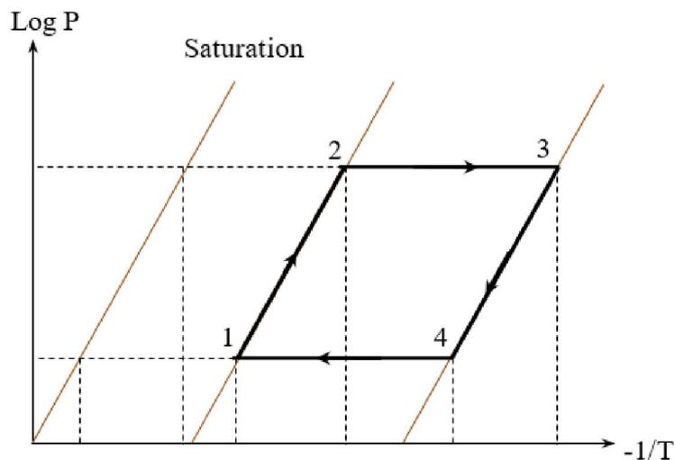
**Figure 2** The ideal cycle in the Clapeyron diagram
